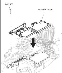
**Note:** Once the Expander mount is installed, reposition the receiver box and wiring on the Expander mount.
