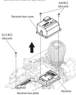
**Note:** After removal of the receiver box cover, carefully lift and move the receiver and wiring to allow installation of the Expander mount over the receiver box plate.
